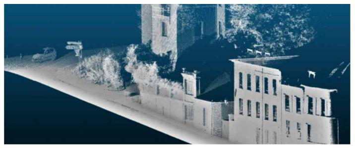
Survey made in Marly le Roi, France, mapping was carried out with **ATLANS-C** and its **Post-Processing Software**, visualized in third party LIDAR software package.
