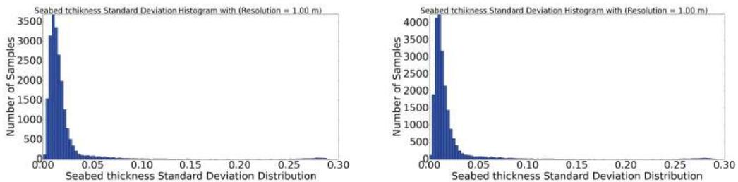
Figure 9: Histograms of SDASN for the four data sets. On the left, data corrected with MIBAC boresight on the right, data corrected with patch test.
