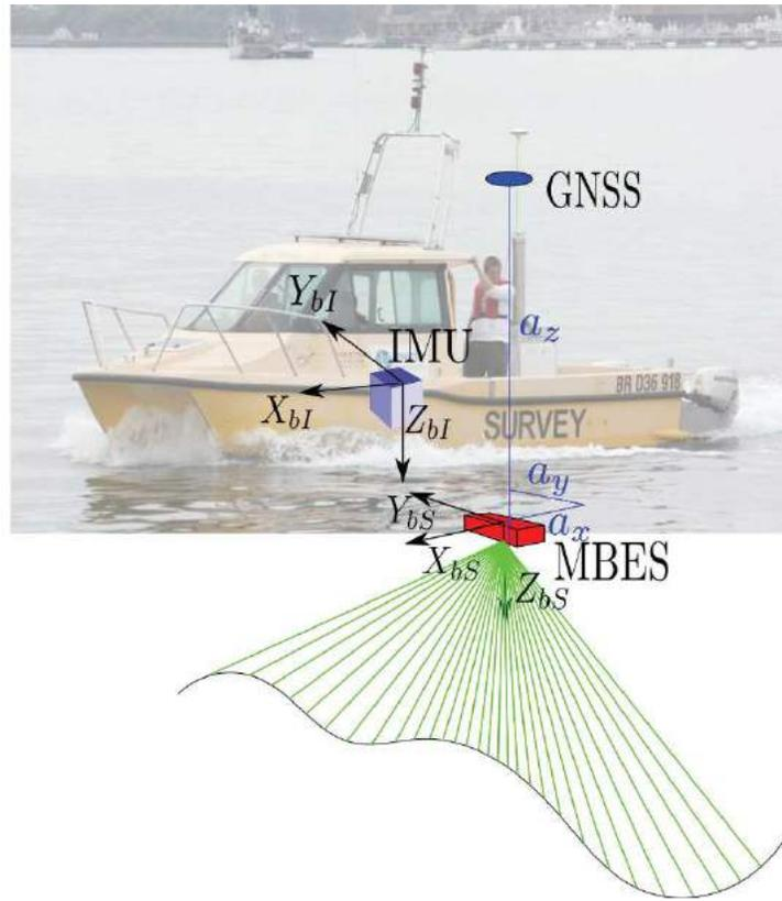
Figure 1: A typical MBES system mounted on a survey vessel. Lever arms components are denoted by  $a_x$ ,  $a_y$  and  $a_z$ . The MBES local frame is denoted by  $bS = (X_{bS}, Y_{bS}, Z_{bS})$ , and the IMU frame by  $bI = (X_{bI}, Y_{bI}, Z_{bI})$ . Boresight angles define the frame transformation from  $(bS)$  to  $(bI)$ , denoted by  $C_{bS}^{bI}$ .
